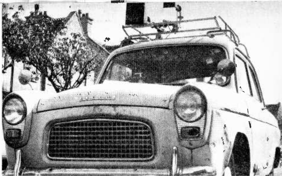
The car in which the prototype anti-collision device, developed by apprentices at B.A.C., has been fitted. The radar transmitting and receiving aerials are seen attached to the roof rack.
