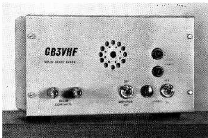
The electronic keying unit employed at GB3VHF, Wrotham, Kent, and designed by G. E. Goodwin, has only one moving part — the keying relay.
