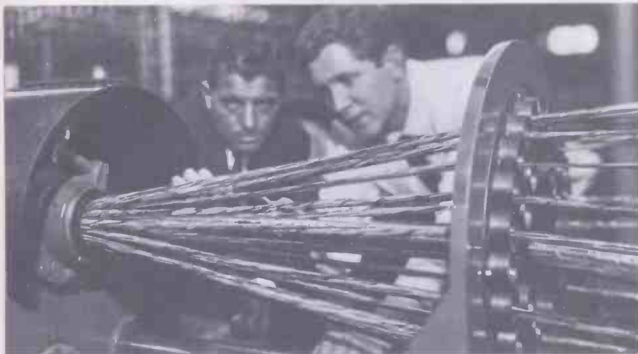
(Above) An 8,000-conductor telephone cable being manufactured at the works of British Insulated Callender's Cables and (left) the finished product. The cable employs "Hyperden" insulation, developed by B.I.C.C., made from cellular polythene 90 \mu m thick giving an increase of 25-pairs-per-cable of a given diameter over earlier methods. The P.O. have successfully laid a length of the cable at Irlam, Lancs.
