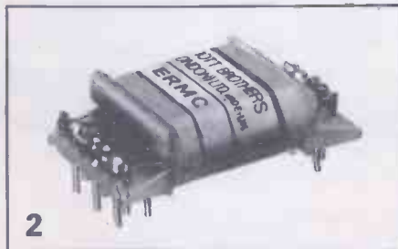
Dry Reed Relay Type ERMC/D/E: Miniature open, shielded and encapsulated styles with up to 5 poles, offering all the advantages of reeds at low cost; standard relays operate from 35mW depending on contact arrangement; electrostatic shielding, high voltage insulation and low thermal types can be specified; life expectancy 10 \times 10^6 operations at full load, contact rating 10VA.
