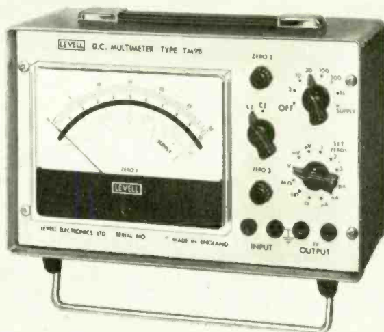
This d.c. multimeter from Levell Electronics measures 0.3 μV to 1 kV in 18 ranges, from 1pA to 1A in 24 ranges and from 0.3Ω to 1000 MΩ in 18 ranges. It incorporates a high-gain, solid-state, chopper-stabilized d.c. amplifier. WW 396 for further details
