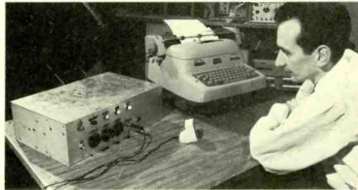
Voice-operated typewriter, showing electronic recognizer on the left. (Standard Telecommunication Laboratories)
