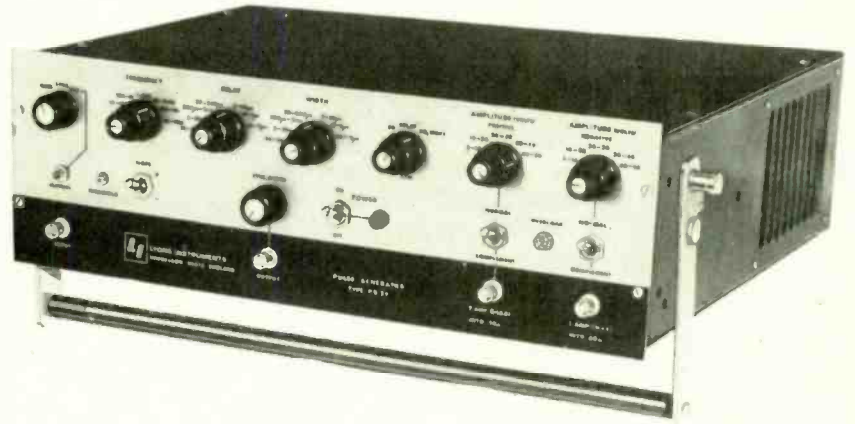
Lyons Instruments new high-power pulse generator (PG 25) provides two outputs of opposite polarity each capable of supplying 1A into 50Ω. Frequency range is 10 Hz to 20 MHz. WW 391 for further details
