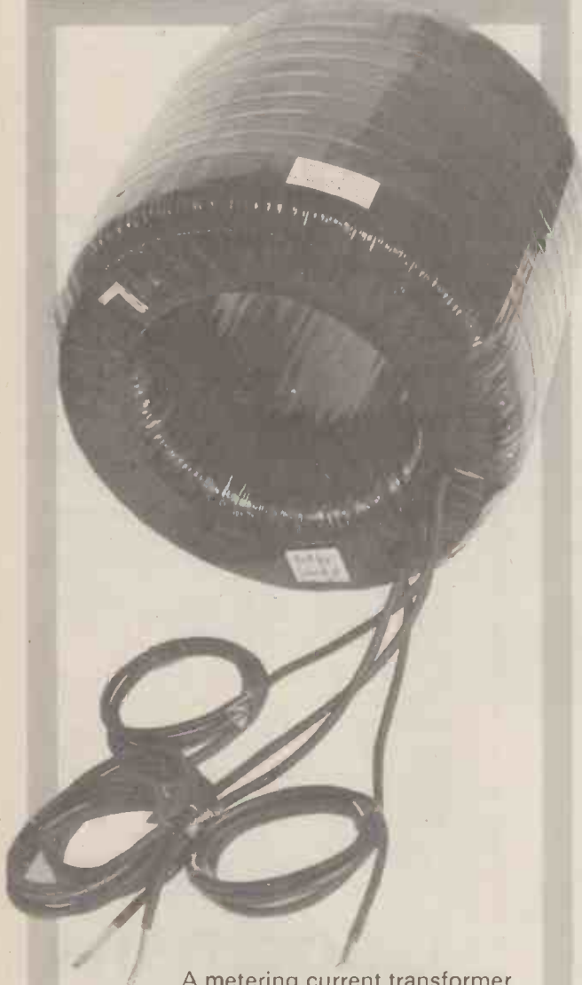
A metering current transformer made by Smith Hobson Ltd., which uses five Telcon Mumetal strip wound toroidal cores.
