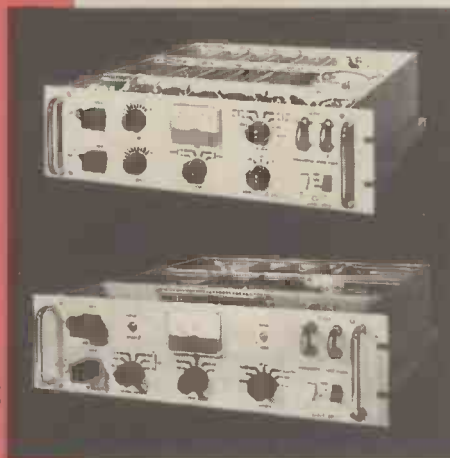
STANFAST MODULATOR UNITS Used with STC h.f. exciter unit Type 4021-D to supply modulated drive to STANFAST amplifiers. Two identical outputs are provided for dualling of service. Type A.1442-A provides SSB, LSB and DSB emissions A3, A3A, A3B, A3J, A7A, and A9B at an output frequency of 100kHz. Type A.1443-A for FSK emissions F1, F4, F6 and on-off keying A1. Nominal output frequency 100kHz.
