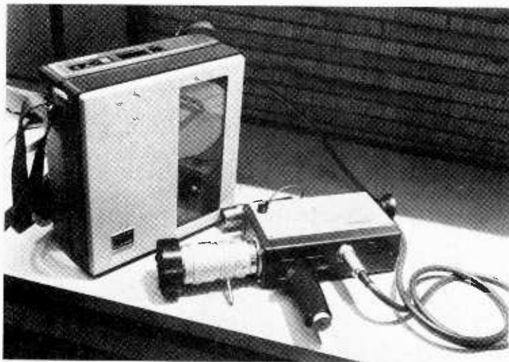
Sony portable video recording unit. The camera has a built-in electronic viewfinder.
