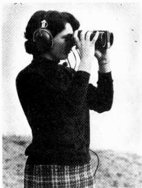
Optical transceiver made from ordinary binoculars.
