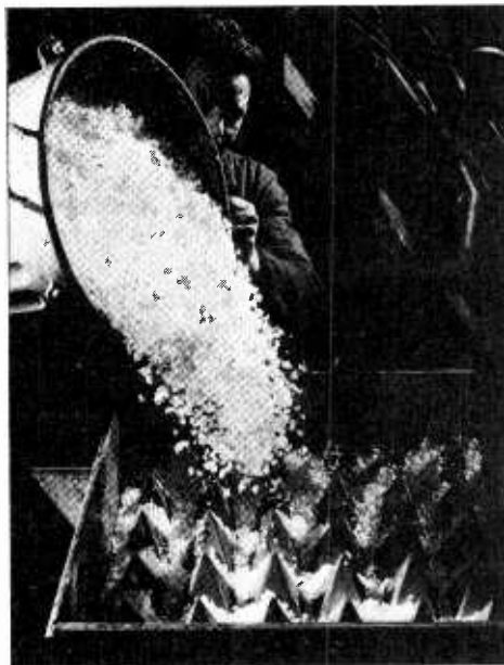
Expanded polystyrene granules being poured into a mould at the components group of Plessey during the manufacture of radar absorbent material. After processing the material will absorb radiation from 0.75 to 30GHz.
