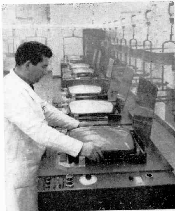
Some of the Thorn-AEI designed "light-houses" in which the faceplate, through its shadow-mask, is exposed to ultra-violet light to form the dots on the phosphor.
