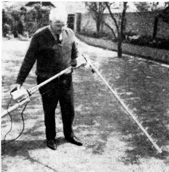
Fig. 4. Author's ultra-fringe, high-gain, rotatable, u.h.f. aerial system (Labgear U-18 aerial and E-5122 booster amplifier, mounted on Channel-Master "Tenna-Liner" rotator).
