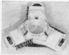
Convergence unit (above) and deflection coil (left) for the Mullard 90° colour television tube.
