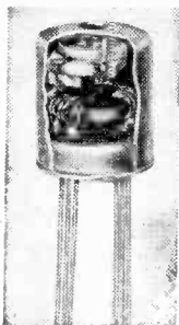
Fig. 1. A typical example of an LC network enclosed in a TO-5 case. The particular item is a phase detector circuit.
