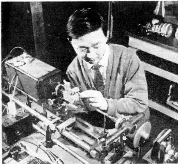
An optical bench at S.T.L. for investigating optical waveguides. A He-Ne laser (left) is used as a light source and the light is launched on to the waveguide through an oil-immersion microscope objective and a crystal of potassium dihydrogen phosphate used for modulation. A photomultiplier is used as a receiver. The fibre guide, although present, cannot be seen since this is less than 400 \mu\text{m} dia.
