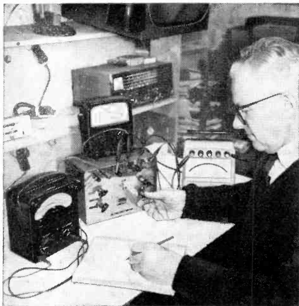
Fig. 3. Author carrying out point-to-point plotting of f.e.t. d.c. characteristics on ordinary laboratory equipment.
