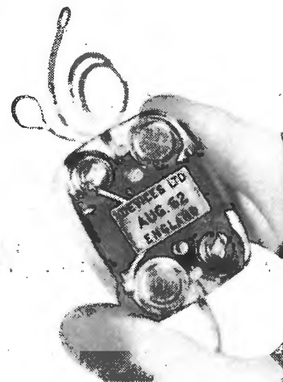
Cardiac "pacemaker," weighing only 100 grams and containing a transistor pulse generator powered by four Mallory cells. An example of Araldite potting.
