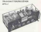
TRANSMITTER A push-pull feed-back oscillator tuneable either side of 445 Mc/s., frequency modulated at 100 c/s by a particularly robust moving coil transducer. Two 955 high frequency acorn valves. Case size only  $3\frac{1}{2} \times 6\frac{1}{2} \times 2$  in. plus  $2 \times 2$  in. dia. for transducer.
