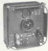
CRYSTAL CALIBRATOR No. 10 CRIBIATOR NO. 10 A crystal controlled heterodyne wavemeter covering 500 Kc/s. to 10 Mc/s. (Harmonics up to 30 Mc/s.) Requires 300 V. 15 mA. and 12 V. 0.3 a. D.C., but can be easily modified for 120 V. and 1.4 V. working. Size  $7 \times 7\frac{1}{2} \times 4$  in. Good condition, complete with valves, crystal, instruction manual and circuit. ONLY 59/6. Post 3/6.
