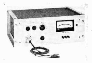
Keithley Model 149 d.c. milli-microvoltmeter.
