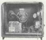
200-250 v. A.C./D.C. Complete with 13 new Brimar valves, latest Fireball turret tuner covering all channels bands I and III (i.f.33-38 Mc/s.). Ferroxcube line output transformer and wide angle 90° scanning coils, ion trap, latest electrostatic focus. All first quality components. Overall dimensions 8×15½in.
