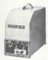
that the same number on the drum will be illuminated by each flash of the lamp. A slowly-varying input voltage will be indicated by a slowly varying number, and interpolation between two partially-visible numbers will give a measure of a voltage between these two numbers. Alternatively, only the nearest number to the actual voltage can be indicated. This is done by making use of an additional set of pulses produced as the numbers pass a phototransistor.
