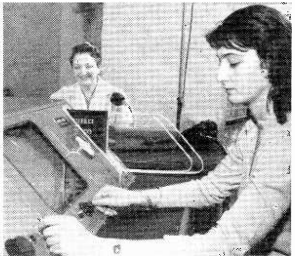
AIR TERMINAL TELEVISION. —Closed-circuit TV equipment has been installed at the West London Air Terminal as an aid to making announcements. The announcement is spoken once only, the announcer appearing on the screens of eight 21-in Pye receivers in various parts of the building, then a "caption" giving the details is screened. The equipment uses a standard Pye Staticon tube camera which covers both the announcer and the bilingual captions, which are inserted in a carrying cradle in the control panel (right). The total cost of the equipment, installed by Audio and Video Rentals, was in the region of £2,000.
