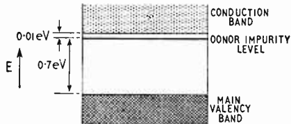
Fig. 6. A donor impurity level is so near the conduction band that at ordinary temperature almost all its valency electrons are found.
