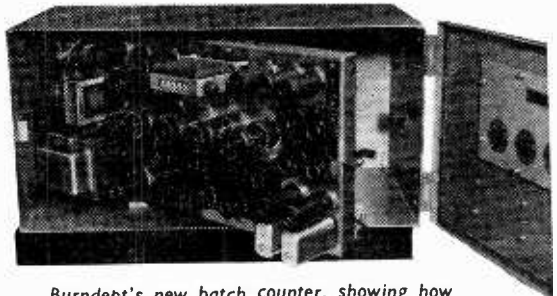
Burndept's new batch counter, showing how the chassis swings out for servicing.
