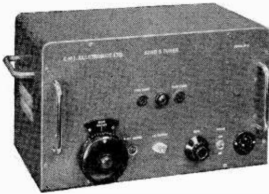
The Band V convertor assembled as a self-contained, screened unit, including power supply.
