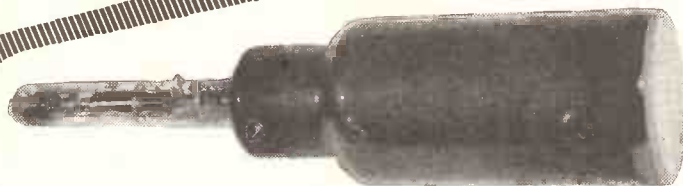
Type G 601-C4 (VCRX 434) High Speed Oscilloscope Tube 30kV Spiral p.d.a. Response 1500 Mc/s Writing speed 10^{10} cm/sec.
