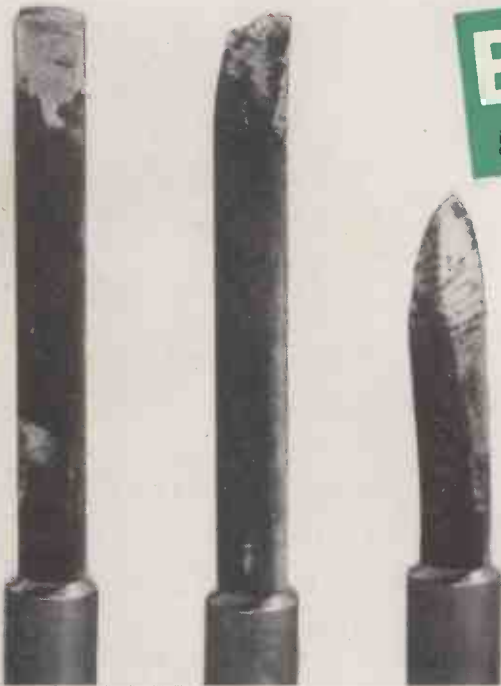
The bit on the left, used with Savbit Alloy, has made 10,000 joints. The centre bit, used for 1,000 joints and the bit on the right for 7,500 joints, were used with a standard tin/lead alloy.
