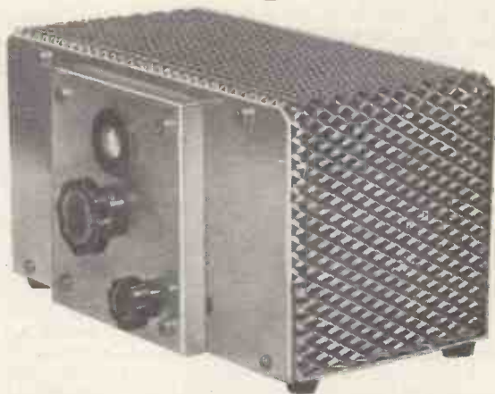
The complete Band-III convertor. The box-like projection on the front of the unit contains a dial mechanism showing the actual television channel to which the convertor is tuned. This is a refinement not dealt with in the text.
