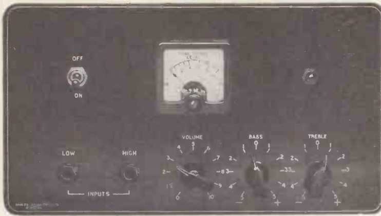
Control panel showing level indicator, main switch, pilot lamp, high and low-level inputs and the volume and tone controls.
