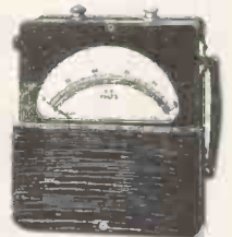
High torque moving coil portable meter. Precision grade to BS.89.
