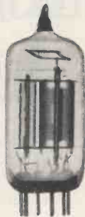
X-ray photograph of modern miniature valve, Osram LN 309.
