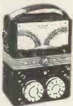
Multi-purpose test set for simultaneous measurement of current and voltage.
