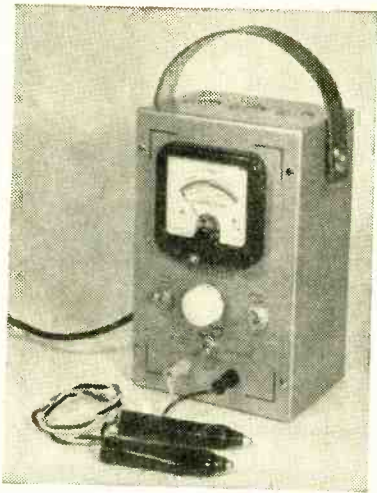
"Trantesta" for testing iron-cored transformers for short-circuited turns.
