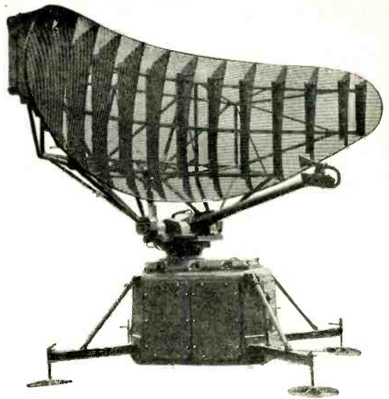
Aerial unit of the 3-cm medium-range Decca Type MR75 surveillance radar.
