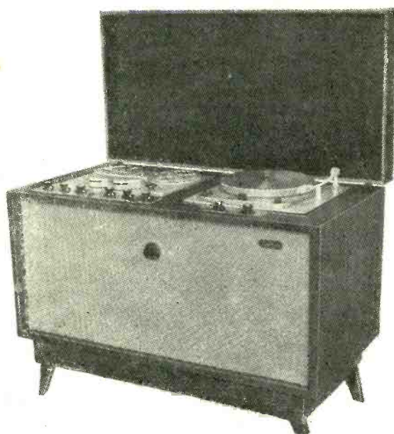
"Spectone" reproducer for "Stereosonic" tape records.
