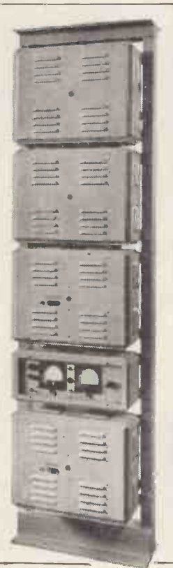
Exchange equipment bay
