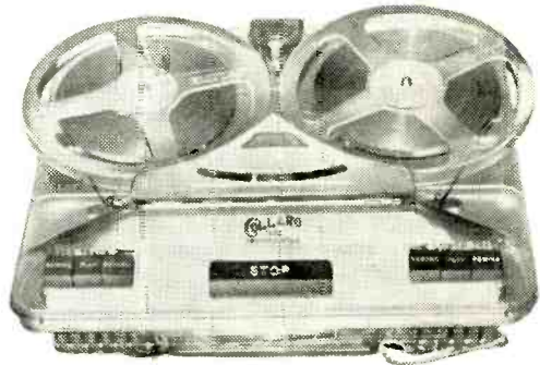
Collaro "Transcriber" tape recording mechanism with and without top cover.
