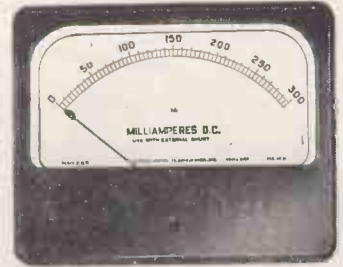
Rectangular panel instruments are available with scale lengths of 2.5", 3.2", and 4.2". These offer the advantage of an increase in scale length of approximately 50% over their equivalent round models, for which they can be used as direct replacements using the same panel fixing holes.
