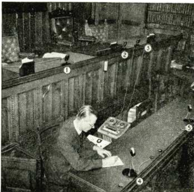
Arrangement of the recording unit and the five microphones in No. 1 Appeals Court.
