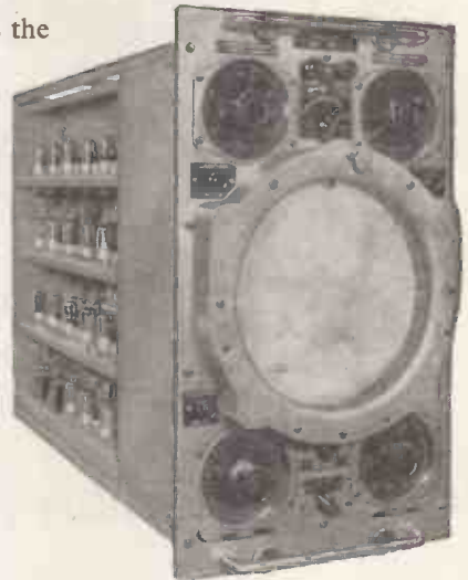
PPI Off-Centre Radar Display Unit designed by B.T.H.; developed in conjunction with B.T.H., leading to substantial quantity production.
