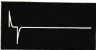
Fig. 3. Waveform of differentiated line sync pulse.
