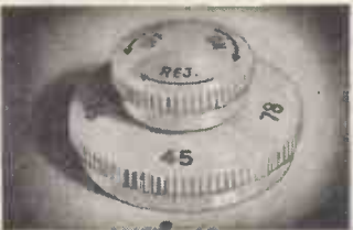
ROTOCAM combined Switch and Speed Control. Concentric plastic knobs working simple connecting rods and slide presetting 33, 45 or 78 r.p.m. speeds. Gives centralised control. Automatically switches off after the last record.
