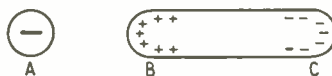
Fig. 1. Typical illustration from old-style book on electricity, showing the effect of a negatively charged body A on a previously uncharged conductor BC when brought near.
