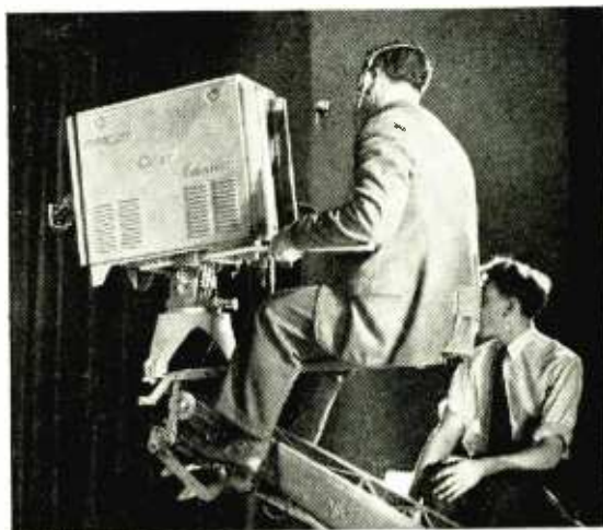
Colour television camera used with the Marconi system referred to in the article. It has only two pick-up tubes (one for high-definition monochrome information and the other for low-definition colour) and is notable for its small size.
