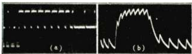
Fig. 2. (a) Video signal of pattern generator during even frame synchronizing period. Negative picture signal. (b) The effect of integrating the synchronizing pulses during the frame synchronizing period. Positive pulses.
