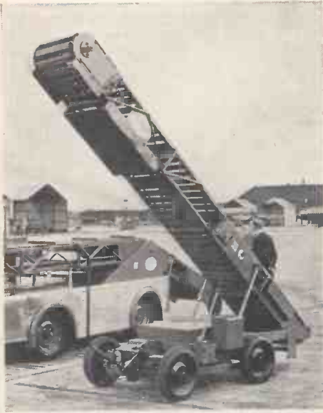
This pedestrian-controlled electric conveyor is easy to handle, has forward and reverse drive, and a maximum delivery height of 11 ft.
