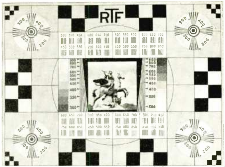
The 300-line test card used by La Radiodiffusion Television Française.
