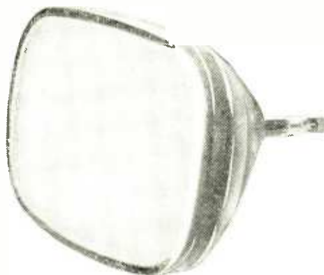
(Left) Ediswan Vapotron valve in its vapour cooling system. (Centre) Mullard 21-inch rectangular c.r. tube. (Right) Two 20-Mc/s quartz crystals in evacuated glass envelope (S.T.C.).
