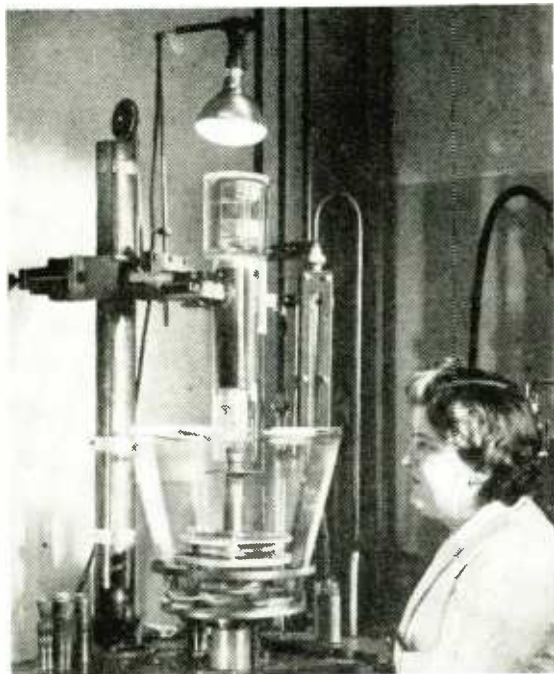
The final sealing-in of the tube with rotating gas flames.
