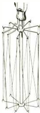
Fig. 2. Typical tungsten filament in vacuum lamp.
