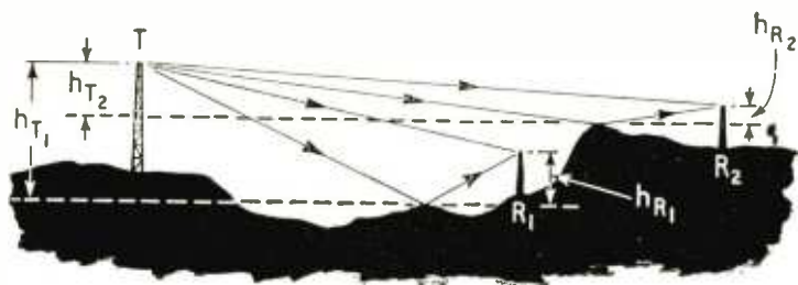
Fig. 2. Transmission over rough terrain, showing relationship between true and effective heights of aerials.
