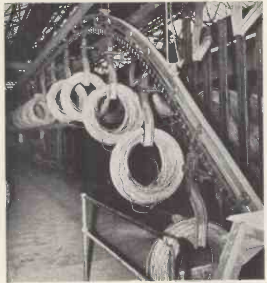
The overhead chain conveyor is here seen in operation with coils of wire. This is a type of mechanical aid which can be adapted to almost any type of industry. One particular advantage of the overhead chain conveyor is that it provides a moving storage system well clear of normal production operations.
