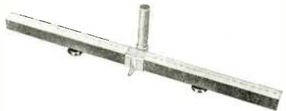
Fig. 2. The complete instrument standing on the rubber suckers. The optical system is housed in the vertical tube.
