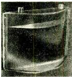
Left: Fig. 2 Experimental plano-convex cylindrical lens partially filled with liquid paraffin.
