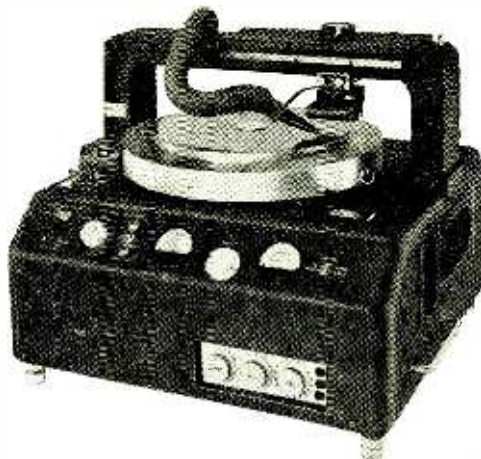
Decca disc recorder, with facilities for servo-controlled automatic variable groove spacing, and (below) transcription from tape to disc by the new M.S.S. Type PMR/2 tape recorder used in conjunction with the Type CLED disc recorder.
