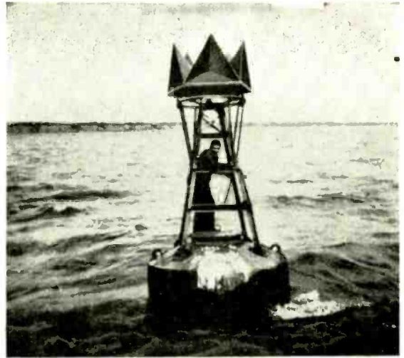
Pentagonal cluster of corner reflectors used in "raflac" trials by the National Research Council of Canada.
