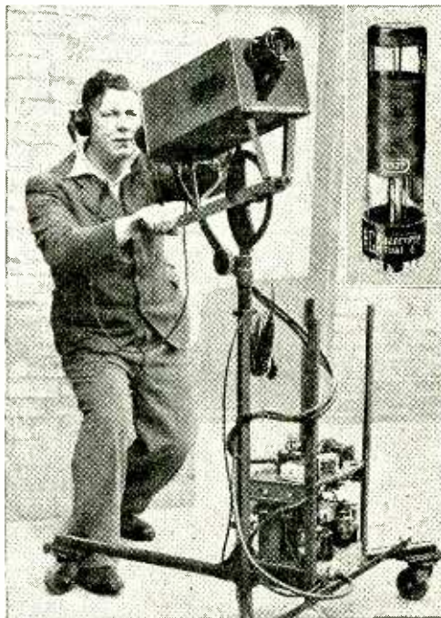
Ivan Howard with the iconoscope camera he has constructed. Inset: Iconoscope tube RCA type 5527.
