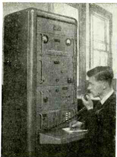
The Ekco V.H.F. equipment installed at the head office of the Southend Waterworks Company. The rack includes a 25-W transmitter, double superheterodyne receiver and control unit.
