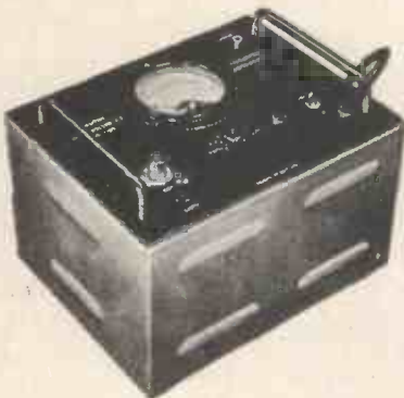
Type 378B/2 1mV to 100V 10c/s to 500Kc/s
