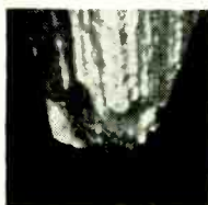
Left: Fig. 3. Fibre needle after playing one side of new 12-in record. Right: Fig. 4. Sapphire point after 250 playings of 250 new 12-in records with a "light-weight" pickup. Weight on point 25 grams.
