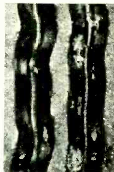
Fig. 2. Record groove after one playing with steel needle, showing abrasions with steel flakes embedded in wall.
