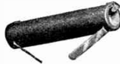
Three type 36EHT35 rectifiers, each only 3" long X 1/2" dia, will, from a peak pulse input of approx. 2,500V obtained from the standard line scanning output transformer, give an output of about 6kV at 100µA, used in the tripler circuit shown on the left.
