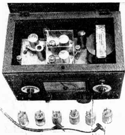
(Left) Tele-Radio V.H.F. converter with coils for the 2-, 5-, 6- and 11-metre bands.
