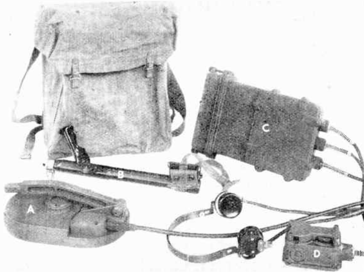
The individual units of the mine detector are shown above. The search shoe A, telescopic handle B, amplifier C and control box D are carried, together with the phones, in the canvas case.
