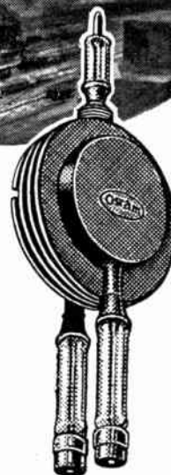
One of the famous Magnetron valves used in many centimetric Radar devices.
