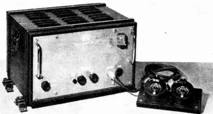
A marine model of the Decca Navigator. World Radio History
