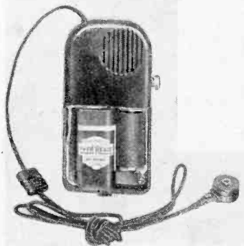
Multitone Type B pocket hearing aid with 10mm. valves and layer-built HT battery
