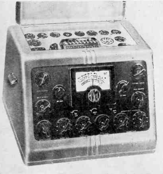
AVO valve tester incorporating an overload cut-out
