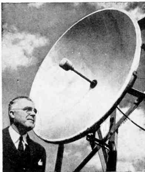
direction—could each provide 270 multiplex circuits. On the left is one of the micro-wave aerials.
