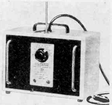
The aerial rod can be seen plugged into its socket adjacent to the cable exit.
