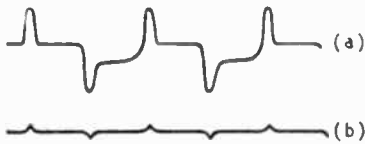
Fig. 1. Variation in voltage across input electrodes (a) without glow-up electrode; (b) with glow-up electrode.
