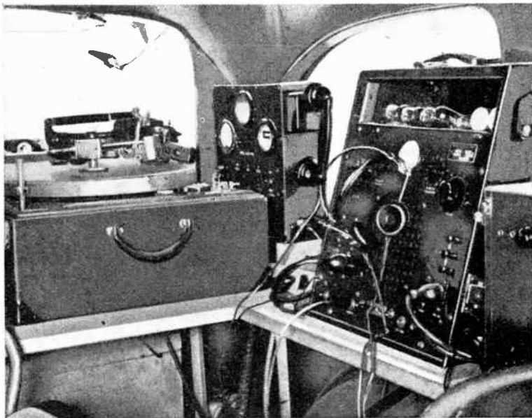
Interior view of the recording laboratory's sound truck, showing one of the 16-in. recorders, control panels, telephone intercommunication link, recording amplifier, etc.
