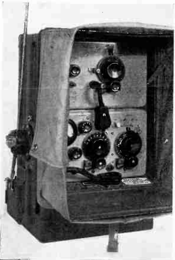
Crystal control of the transmitter frequencies (1.75—2.9 Mc/s) is provided in the No. 68 P transmitter-receiver (above).
