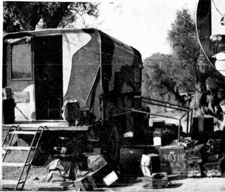
The repair and maintenance of the Army's telecommunications equipment—the collective term used for radar, wireless and line gear—is the responsibility of R.E.M.E., and the illustrations show a repair workshop of a mobile wireless detachment which provides repair facilities behind the front line. These mobile workshops, which have proved their value in fast moving warfare, handle all but the simple repairs and adjustments to the wireless and line equipment in the hands of units in the front line, which is undertaken by men of Royal Signals. Equipment beyond repair in the combat zone is returned to the large static telecommunications workshops set up in the various theatres of operation.
