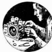
SPECTRUM ANALYSIS The exact composition of materials used in the manufacture of WESTINGHOUSE METAL RECTIFIERS is determined by spectroscopic apparatus, and spectrograms are prepared of specimens as required. The illustration shows the arc method of excitation in use.
