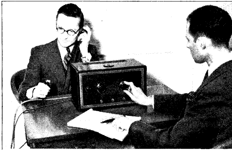
This photograph, taken by courtesy of the Hearing Aid Department of the Western Electric Company, shows a patient undergoing an air conduction test with an audiometer. This instrument, which is also provided with facilities for bone conduction tests, can be set for any frequency up to 10,000 c/s, and enables the operator to plot an audiogram showing the extent and characteristics of a patient's hearing loss at various frequencies.
