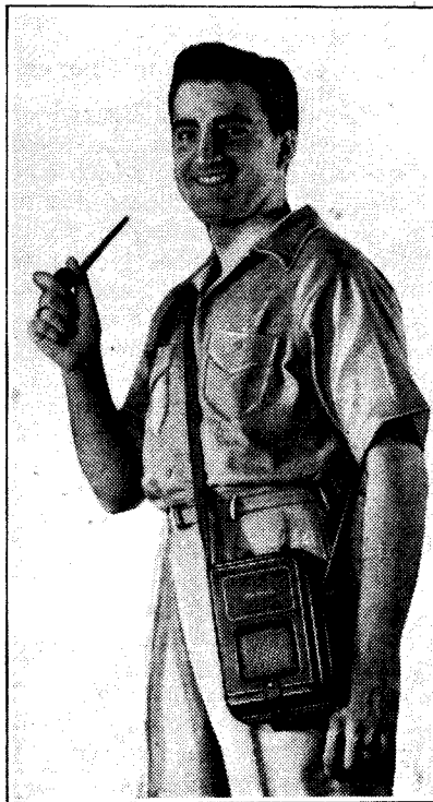
Small set, large aerial. An ingenious method of increasing the pick-up of the frame aerial is embodied in this miniature American portable. The wires of the frame are woven into the webbing carrying strap. Incidentally, the latest American miniature valves for sets such as this are designed to work on 45 volts HT.
