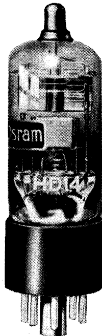
Another example of an "all-dry" valve—an Osram top-capped diode-triode.
