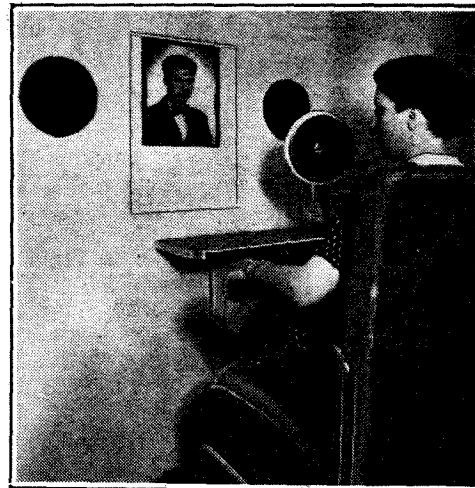
COMFORTABLY ENSCONCED IN AN ARMCHAIR before the television-telephone apparatus in Munich which has just been linked with Berlin. In this official photograph the image on the cathode-ray tube shows much more than in actual practice when the head is larger and the image is cut off just below the collar. Note the loud-speaking telephone in front of the speaker.
