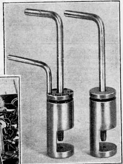
CHASSIS SUPPORT. This adjustable steel cradle, of American manufacture, is arranged to give easy access to any part of a radio chassis. The base may be extended up to 26 ins., and the clamps, though holding the chassis firmly, allow for tilting the angle best suited to the work on hand.
