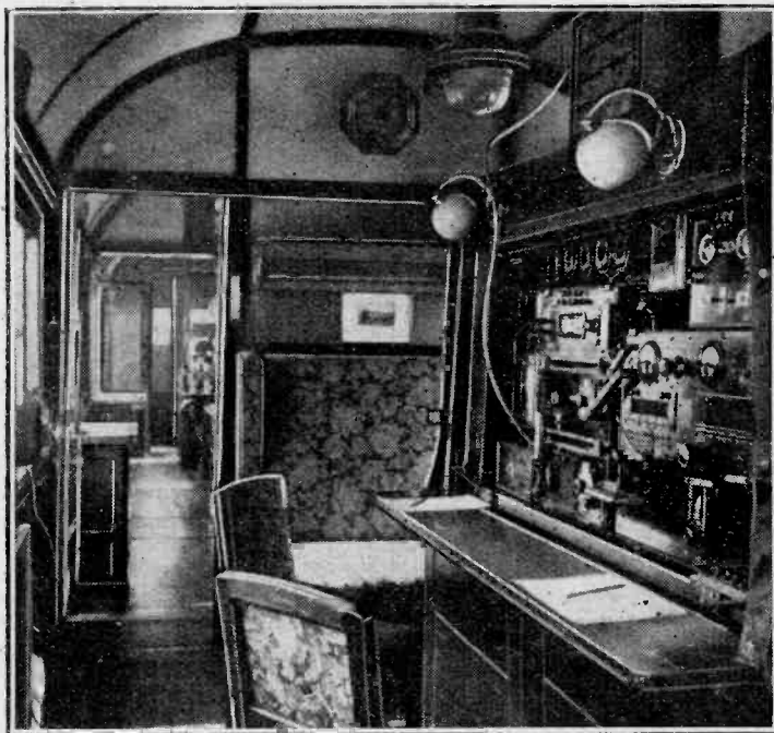
TRACKING INTERFERENCE on the German State Railways; this photograph shows part of the measuring apparatus installed in a special rail coach with the object of investigating electrical interference.
