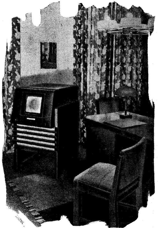
The Telefunken television receiver requires an aerial of only 10 feet to provide adequate reception. A picture of 18 x 22 cms. is sufficiently brilliant not to require a darkened room for looking-in.
