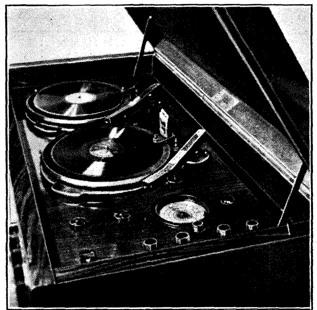
Volume contrast expansion is available for radio reception as well as for the output from the two piezo-electric pick-ups. The controls include a flexible system of bass and treble compensation.
