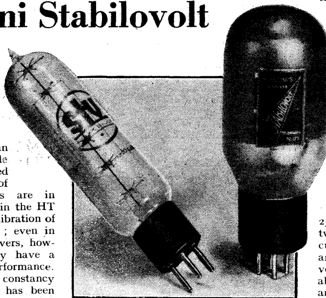
The type H85-255/80 barretter is shown on the left and the STV 280/80 Stabilovolt tube on the right.
