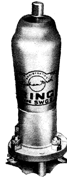
A Graham-Farish short-wave SG valve. The base is of low-loss material, and inter-electrode capacity is reduced by leading out the grid connection to the top cap.
