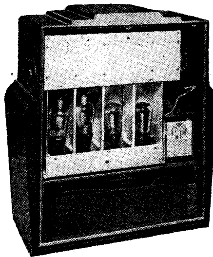
A fine example of a 1930 self-contained 2-HF receiver, the Pye portable.
