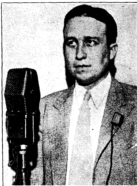
"RIBBON" MICROPHONE FOR COAT LAPELS. It is claimed for this "personal microphone," a product of the R.C.A. Victor Company, Camden, N.J., that it sacrifices none of the technical qualities of the large studio instrument seen on the left.
