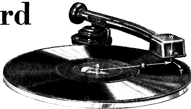
Fig. 2.—From measurements of the retarding torque T , the needle pressure W , and the radius of the groove R the coefficient of friction of the record material can be calculated.
