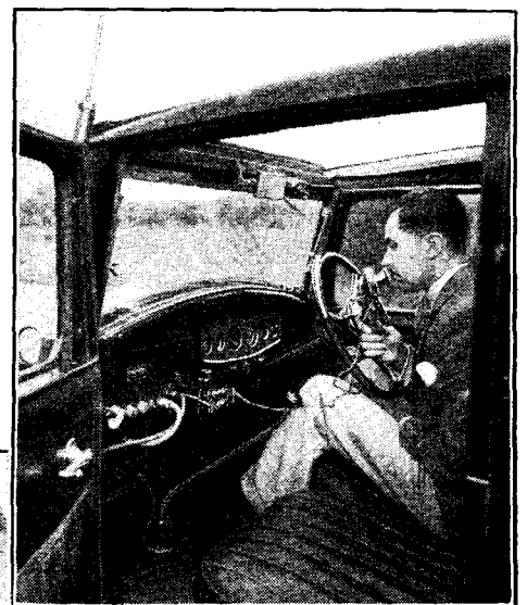
POLICE WIRELESS. A Marconi engineer testing a new police wireless transmitting and receiving equipment installed in a saloon car. The receiver can be seen next to the dashboard, which carries the control switches, and the transmitter is below.
